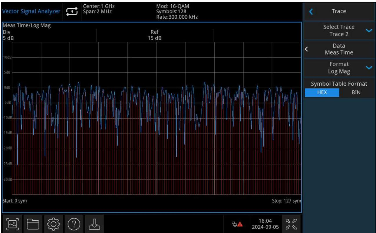
Figure 3-2 Logarithmic Amplitude Format
