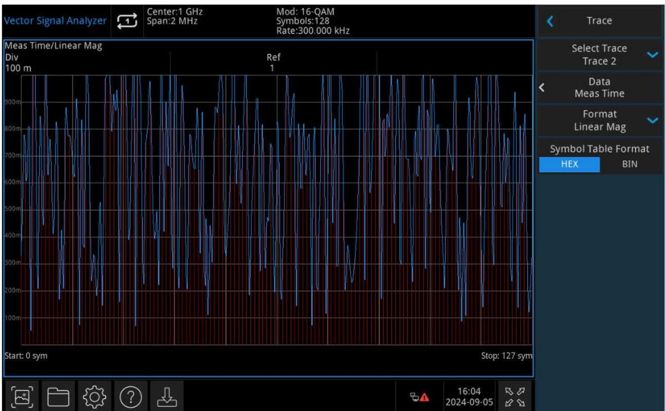
Figure 3-3 Linear Amplitude Format
