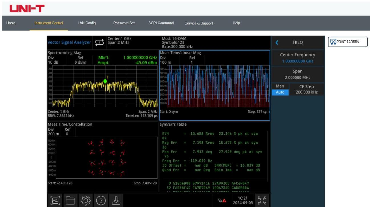
Figure 3-14 Web Instrument Control
