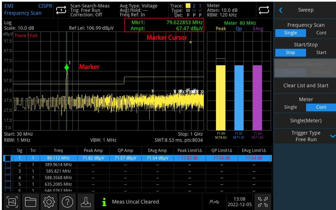
Figure 3-2 Reading of Marker Cursor
