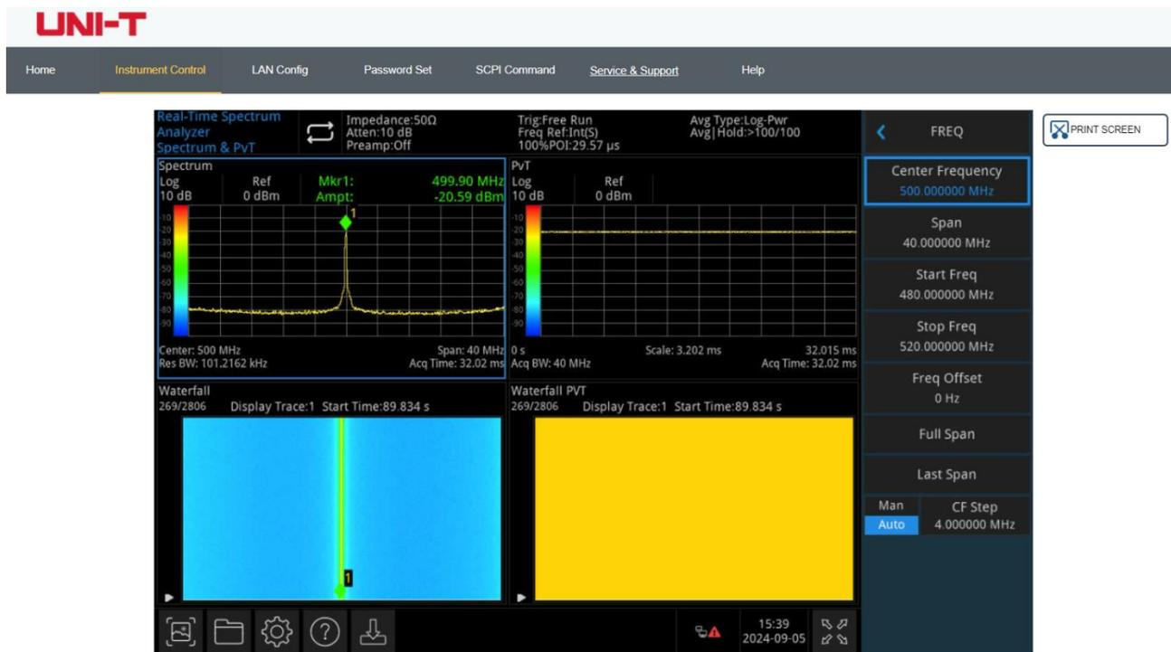
Figure 3-20 Web Control for Instrument
